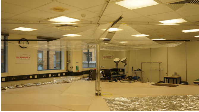
Fig. 33: Dragsail: Deployment Test. With EQM unit.
