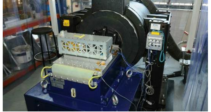
Fig. 35: Dragsail: Vibration EVT Testing. With EQM unit.
